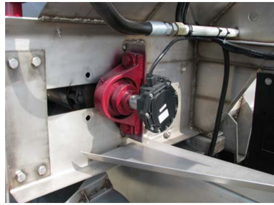
Shaft mounted rate sensor for automatic rate control.
