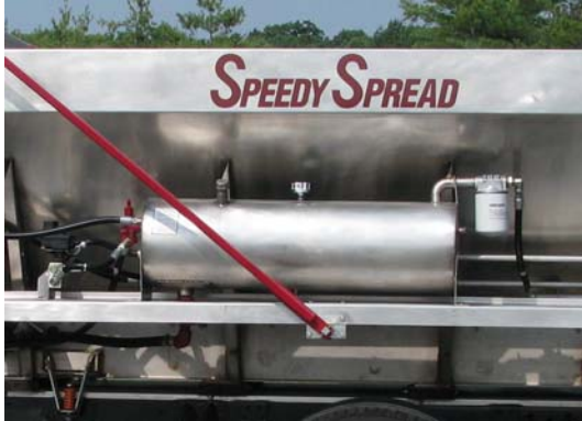
Large capacity stainless steel hydraulic oil tank w/ shut off valve and return filter
