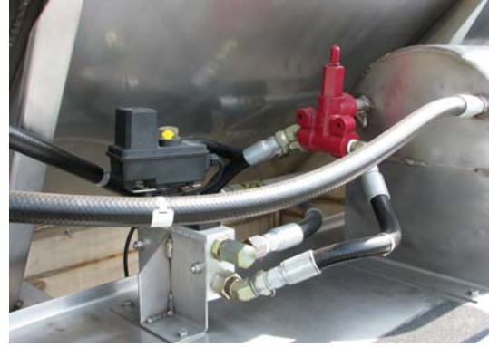
Hydraulic control valve for conveyor control and in line pressure relief valve
