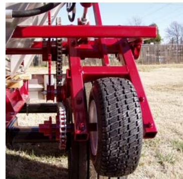
Hydraulically operated press wheel w/ easy switch from fertilizer to lime.
