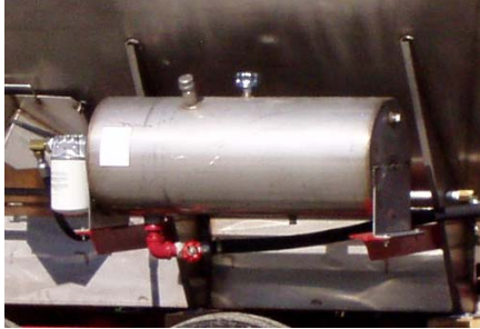
Large capacity stainless steel hydraulic oil tank w/ shut off valve and return filter
