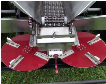
Bottom mounted gearbox driven 20" spinner plates and stainless steel spinner blades.
