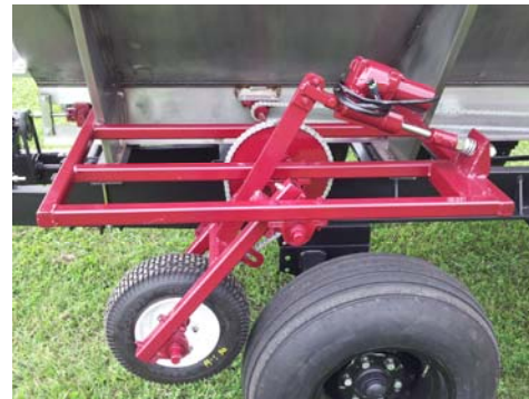
Heavy duty tubular frame with 6500 lbs tandem torsion axles and truck bed liner coating on frame.
