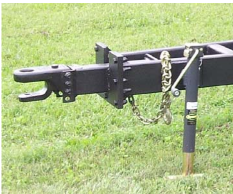
Heavy duty forged steel adjustable hitch and safety chain.
