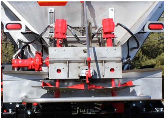
Top mounted hydraulic motors with 24" spinner plates and stainless steel back plate and bumper
