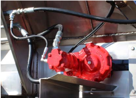
Hydraulic conveyor drive assembly with 6 to 1 Rawson gearbox system
