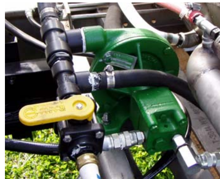
Hydraulic Driven Tank Rinse Pump
