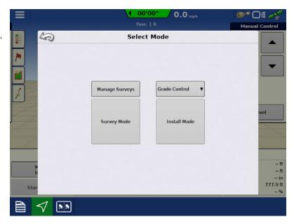
**"Up" and "Down" buttons**—used to raise or lower the cutting edge of the machine before engaging automatic control.
