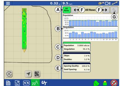
operating at the highest and lowest levels for singulation and population. The screen also shows the averages for specific drive sections.
