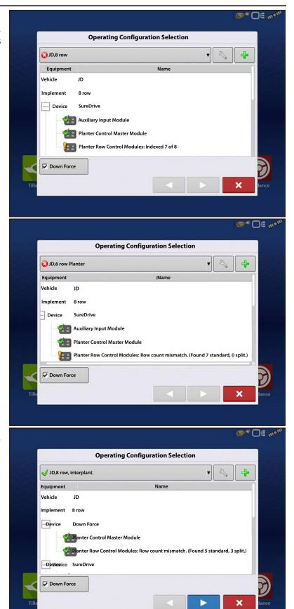
How the Field Select Wizard should appear when all RCM modules have been found on the CAN Bus, properly indexed, and properly assigned to each of the rows.
