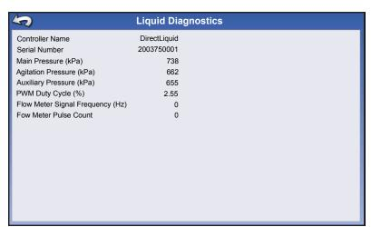
The Liquid Diagnostics screen includes the Active Controller Name and the Serial Number of the module. Other information provided includes the Main Pressure, Agitation Pressure, and Auxiliary Pressure. These raw sensor readings are shown in kilopascals (kPa).
