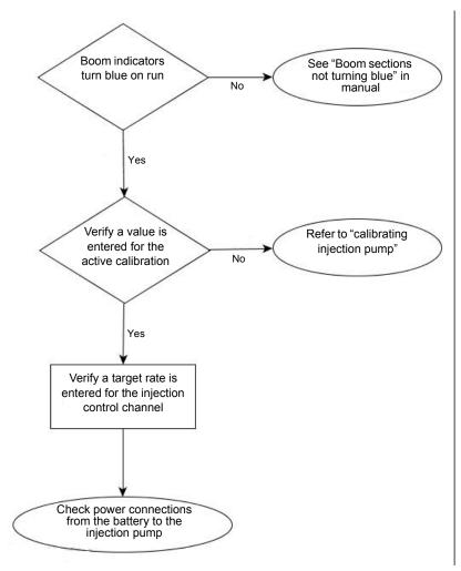
Power can be checked at multiple locations. First is the connection at the Injection module where the battery power cable plugs in. The second location is the output connection found on the injection module. The third is found at the 2 pin weather-pak tower found on the injection cable PN: 4000851-3. See table below.
