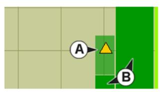
When the Map screen is running in a Zoom Detail view, **instantaneous coverage (A)** is shown automatically. However, there is a time lag between when grain enters the combine through the Header and is logged by the Flow Sensor in the Clean Grain Elevator. Because of this time lag, the instantaneous coverage is shown on the Map screen as a lighter color than **coverage that has been logged (B)** by the display.
