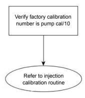
The injection module requires that a pump calibration be performed before actual application can occur. The calibration number found on the tag of the injection pump's digital speed sensor needs to be divided by a factor of 10 before entering it as the factory calibration number. If the factory cal number is entered wrong, the pump calibration routine will not finish due to a high application error.
