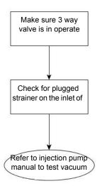
The injection pump has a vacuum switch that is used to warn operators of any restriction at the inlet of the pump. The sensor is a normally closed switch that opens if a restriction is encountered in the injection system. A warning will be displayed for the operator if the vacuum switch opens due to restriction. See table below for pin locations. The operator can test the system by unplugging the sensor, which will trigger the warning. If the operator jumps pins A and C, the warning will end.
