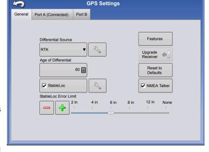
– even when your correction signal is temporarily lost – by seamlessly transitioning to the next available signal source. When the signal is restored, the system will then transition back to the higher accuracy source, eliminating position jumps.
