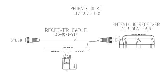
**NOTE:** The Phoenix 10 is powered by a 9 - 16 VDC negative ground system.
