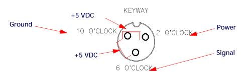
**NOTE:** If a +5 VDC voltage reading is not present, disconnect the flow sensor cable. If the speed reading is restored, refer to the Testing Flow Meter Cables section on page 48 to test the flow meter cables.
