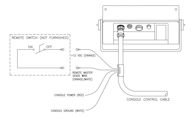
An optional remote switch may be installed if the console is mounted in a location that is not easily accessible. A remote switch may include a foot switch or a toggle switch on the joystick. To utilize the remote switch, the master switch on the console must be turned off. The master switch on the console can be used again once the remote switch is turned off. Refer to the figure above to install the optional remote switch.
