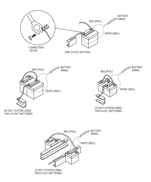
turned OFF, the system will continue to draw 0.25 milliamperes of current to maintain information stored in the console computer, draining the battery.
