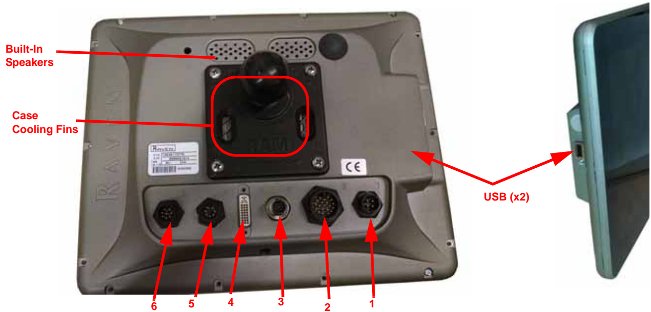
FIGURE 5. Viper 4+ Ports and Connectors
